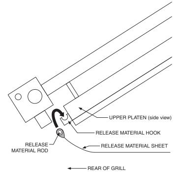
Holding the bottom of the release material sheet in place, gently pull the sheet toward the front of the platen.
